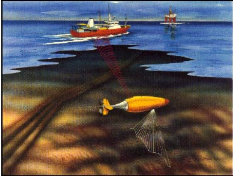
Fig. 9. 'Hugin' is a semi-automatic under-water vehicle able to perform a sonar survey of 36 hours. The data can be transferred via an acoustic link to the mother vessel and displayed as the survey proceeds.
